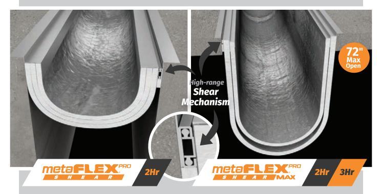
▼ Same great features and performance of the MetaFlex Pro with the addition of a mechanized flange. along one side allowing for up to ±100-percent horizontal shear movement; designed for applications requiring lateral shear. MetaFlex Pro Shear MAX extends the MetaFlex Pro Shear design to 72" max open with ±100-percent multi-directional movement; ideal for locations of high seismic activity
