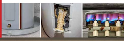
Standard gas and electric water heaters form deposits that inhibit heat transfer.
