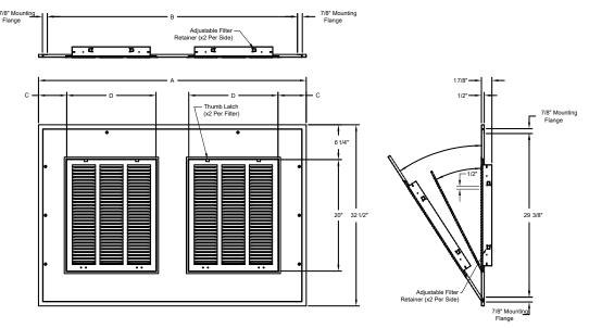
Note: This submittal is meant to demonstrate the general dimensions of this product. The illustrations are not meant to detail every aspect of the product. Drawings are not to scale.
