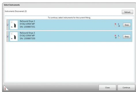
**C** To assign each hearing aid to either the right or left ear, select **Beep** (you will hear a tone), then select the radio button corresponding to the appropriate side. Select **Continue**. If fitting a Receiver-in-the-Ear model, select the appropriate receiver power level, then select **Continue**. Then, select the appropriate Vent Configuration or Dome Size for each hearing aid and select **Continue**.
