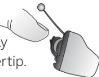
2. Remove protective sticker from battery and wait 2 minutes before inserting the battery into the hearing aid to allow full activation of the battery.
