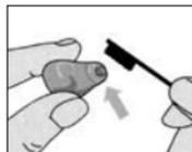
2. Insert the threaded end of the wax filter tool into the used wax filter, and rotate clockwise.
