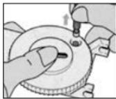
7. Press the new filter to the canal tip of the hearing aid. Move the tool gently side to side and pull it away from the hearing aid.
