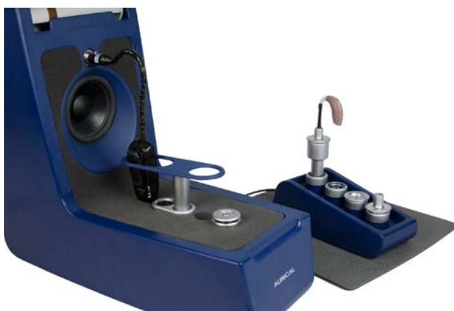
Figure 5. Positioning of the hearing instrument outside AURICAL HIT in the external accessory module. The Multi Mic is positioned on the elevation plate in AURICAL HIT.
