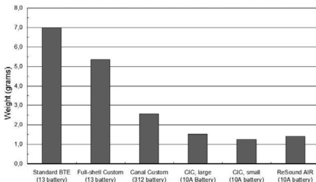
Figure 1. Weights (grams) for six different typical hearing instrument options including required components (i.e. tubing, earmould, battery).
