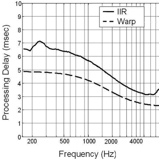
*Figure 2. Processing delay across frequency for Warp and IIR processors.*
