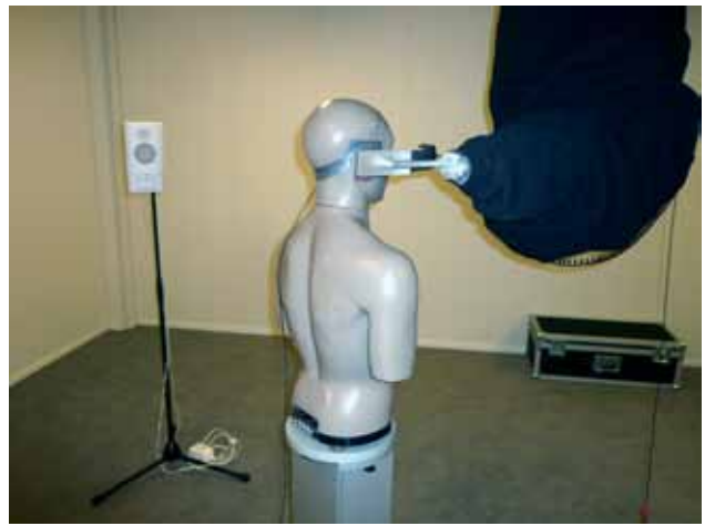
Figure 5. Robotic arm lab testing of DFS Ultra with a KEMAR manikin.
