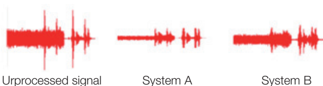
Figure 1. Modulation-based noise reduction systems can decrease noise levels, but can also affect gain for speech. Waveforms recorded with two different systems show reduction of peaks of speech, which could impact both speech clarity and audibility.
