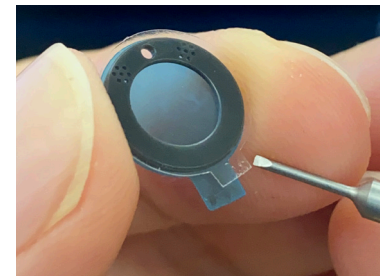
4. New filter rings have a clear sheet on one side and blue sheet on the other. Have the clear sheet facing up.
