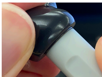
11. Press the cylindrical tool firmly to make sure the filter ring is securely attached to the faceplate.
