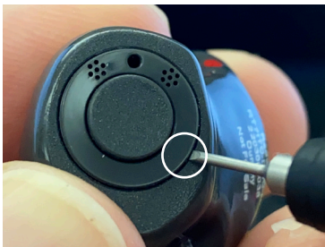
1. Push in the tool in the space between microphone filter ring and faceplate shown in the picture above.
