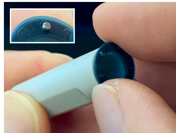
7. Place the filter ring on the gray cylindrical tool. Make sure the hole of the filter ring is placed through the metal pin.
