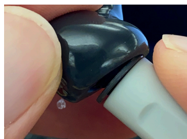
10. Align LED and metal pin then carefully attach the filter ring to the hearing aid.
