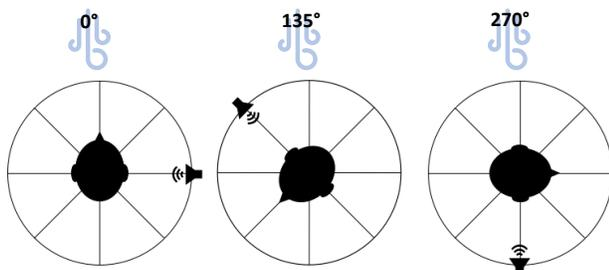
Figure 2. Illustrations of how the KEMAR was rotated relatively to the exhaust of the wind tunnel to create the three incidence angles. The loudspeaker was always placed at 90° azimuth.
