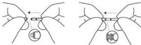
the sound outlet until the outer ring is touching the sound outlet. Pull the tool straight out – your new wax filter will remain in place. Re-attach your dome or a replacement dome.
