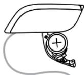
4. Gently close the battery door. If it doesn't close easily, check to see if the battery is upside down.
