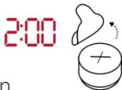
3. Insert the new battery with the positive side (flat side) in the correct position, as shown.
