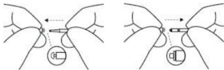
2. **Insertion:** Insert the other end of the tool into the sound outlet (the end with the replacement filter). Gently press the replacement straight into
