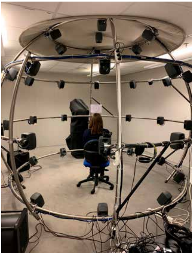
Figure 2. Test environment with 39-speaker playback array.
