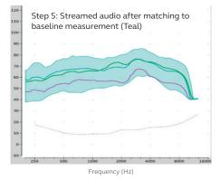
Note: Audioscan Verifit 2 Speechmap screenshots show measurements using ReSound LiNX Quattro RE962 Hearing Aids with all advanced features turned off, using ISTS test stimulus. Apple iPhone 8 was the smartphone used for the streaming portion of the testing.
