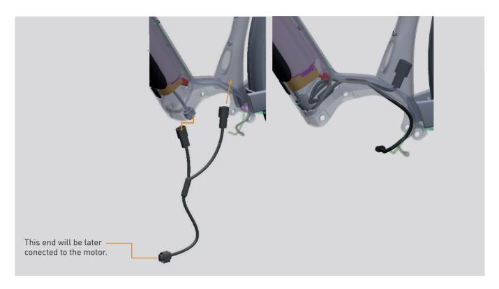
Mount the rail on to the frame with the pre-assembled brackets. Route the cable in and connect with the other end of the Y-Cable.
