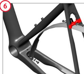
Screw the fender onto the bottom bracket (M5 \* 10 mm screw, M5 washer) and screw the slot onto the seat stay bridge (M5 \* 30 mm screw, 2 x M5 washers, M5 nut).
