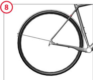
The fender should be the same distance from the tyre along its entire length. In the worst case, too small a clearance the fender can chafe the tyre. If the fender fouls the seat tube on small frame sizes: glue more protective stickers on the seat tube.
