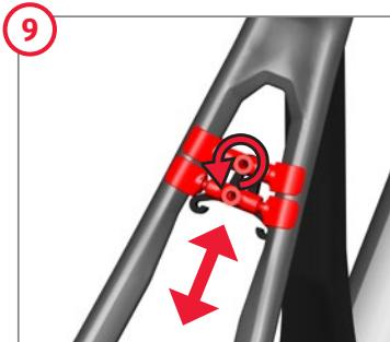
The distance of the mud guard can be adjusted through the position of the bridge and the plastic hook. By turning the central part, the ends are moved by the thread and can be adjusted for different frame sizes.
