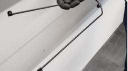
**6** Slide strut fixtures onto the mudguard stays.
