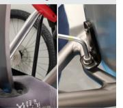
(B) Centre-punch the previously applied markings and drill out using a cordless screwdriver and drill bit (HSS 6mm).
