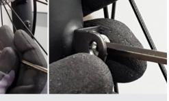
**3** Fit the bracket to the mounting using the bolts and washers provided for this purpose.
