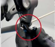
Mount the luggage rack on the dropouts using the M5x18mm bolts and standard M5 nuts provided and a 4mm Allen key with the prescribed tightening torque.
