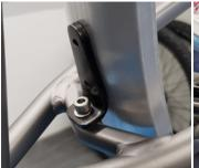
Fit the bracket loosely to the mudguard and seat stay using the M5x12mm nut and bolt. Secure the bolts using medium strength.
