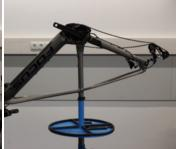
Mark the top of the two holes of the loosely mounted bracket using a sharp object (such as a screwdriver).
