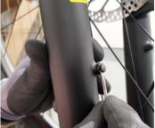
2 If necessary, remove any plugs from the mudguard holder.
