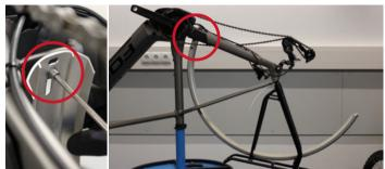
First fit the rear-wheel mudguard using a 4mm Allen key and the M5x10mm bolt and plain washer provided loosely and only to a single point on the engine mount.
