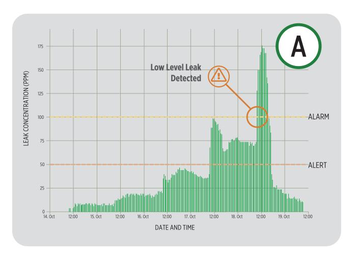
One classic example of a refrigerant leak was recently witnessed at a large US supermarket chain's store. Usually, these 'volcano leaks' start as a very small pin-hole leak that slowly grow unnoticed over time. Eventually, the leak grows so much that it 'erupts', releasing the circuit's remaining refrigerant charge, with the refrigeration equipment failing along with other consequent damage.
